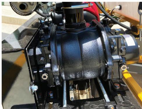
**MAXIMUM LONGEVITY.** The positive displacement roots blower comes standard on all models and features dual oil bath lubrication.
