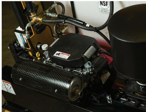
**ENGINE CAPABILITIES.** The VSK25-100G is powered by a 24 hp (17.9 kW) Honda petrol powerpack.
