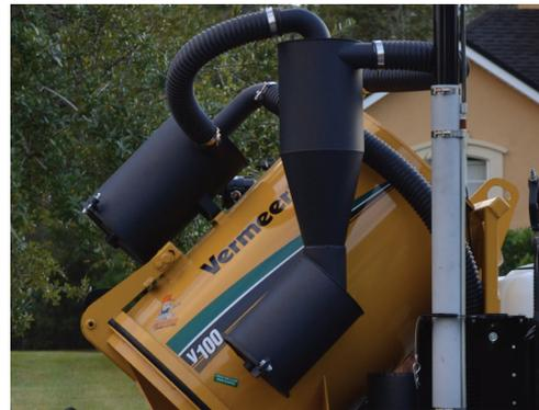
**MAXIMUM SYSTEM PROTECTION.** The VSK25-100G features a three-stage filtration process includes a cyclone separator and a 2-micron poly filter.
