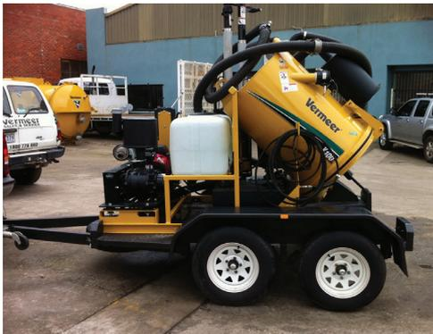
**IDEAL FOR SMALLER JOBS.** The VSK25-100G is ideal for small hydro excavation jobs, such as 'last mile' Fibre To The Premises (FTTP) construction and valve box cleanout.
