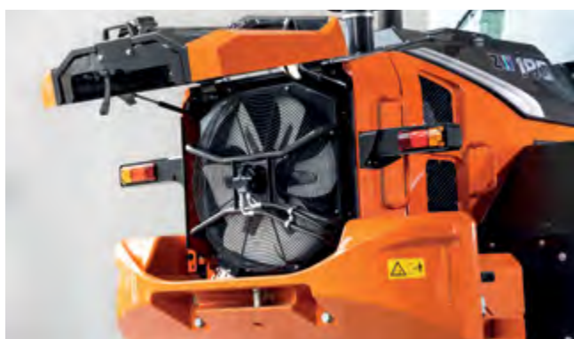
Intelligent fan operation system prevents radiators clogging.
